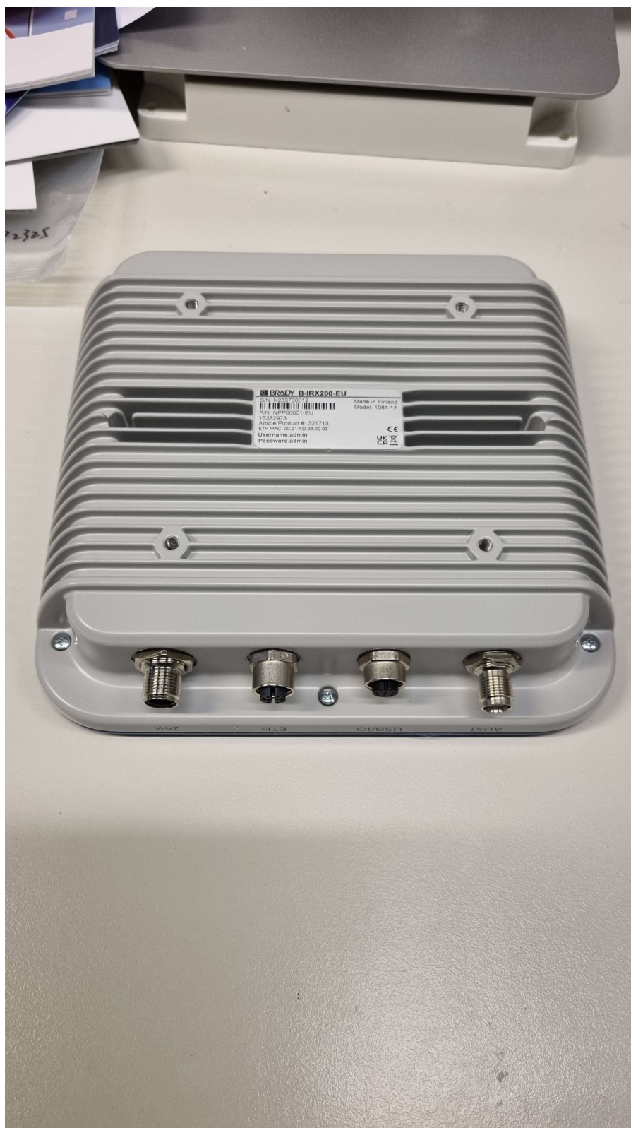
Picture 3. IRX200 connectors view. XA20 antenna have only AUX RP-TNC connector
