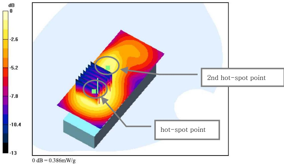
**2. If DASY 4 System fined secondary maxima 2 dB and a peak SAR value greater than 0.5 W/kg, it perform the test about 2nd hot-spot.**
