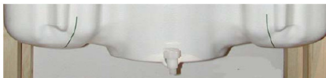
Figure 7.2 SAM Twin Phantom shell
