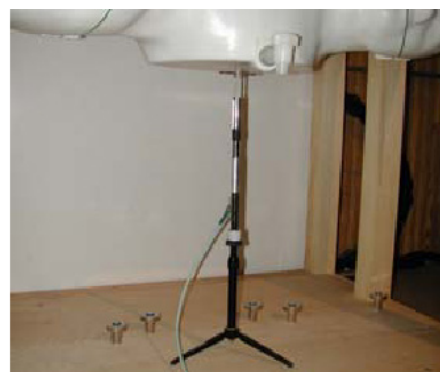
Figure 12.1 Dipole Validation Test Setup
