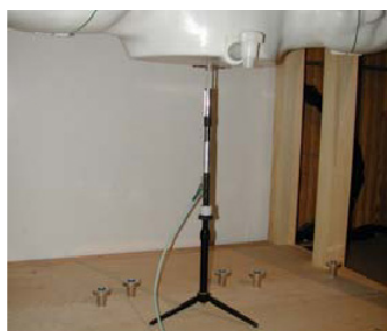
Figure 12.1 Dipole Validation Test Setup
