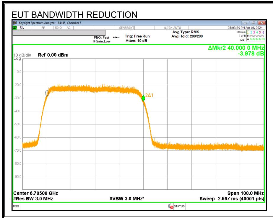
With the Incumbent Signal set to the Upper Edge  $f_{c3}$  the EUT continues to operate at a reduced 40MHz bandwidth.
