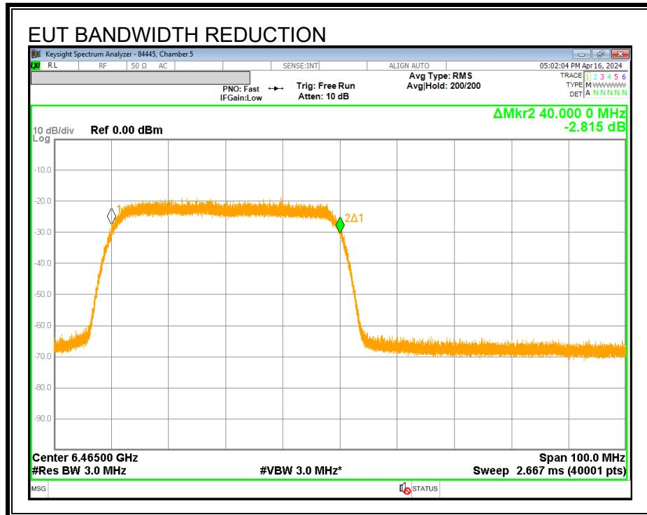
With the Incumbent Signal set to the Upper Edge  $f_{c3}$  the EUT continues to operate at a reduced 40MHz bandwidth.
