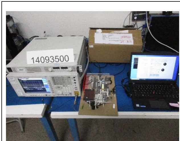
RF ANTENNA PORT CONDUCTED
