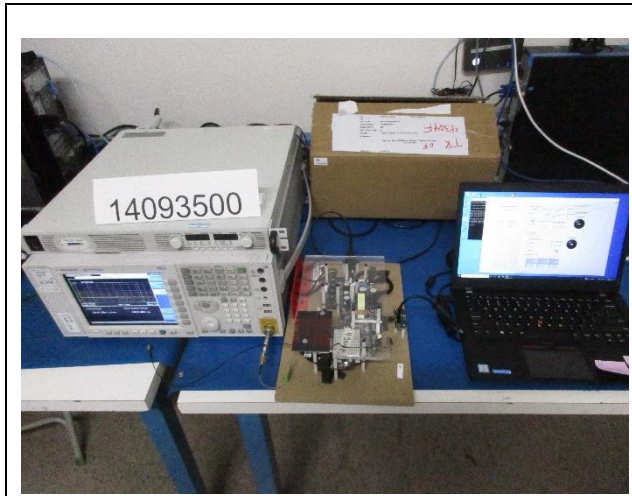
RF ANTENNA PORT CONDUCTED
