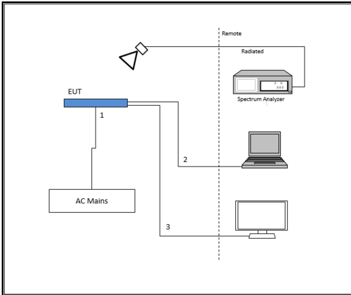
**SETUP DIAGRAM FOR RADIATED ABOVE 1GHZ TESTS**
