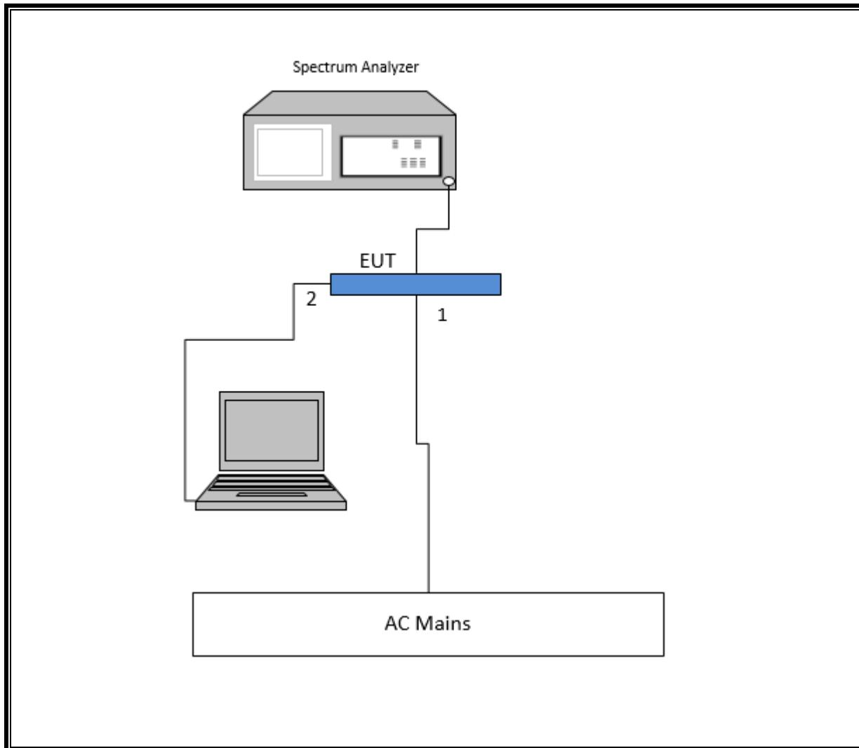
**SETUP DIAGRAM FOR AC LINE CONDUCTED TEST**
