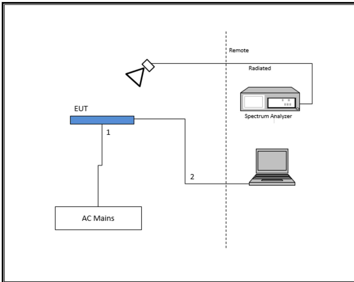
**SETUP DIAGRAM FOR CONDUCTED TESTS**
