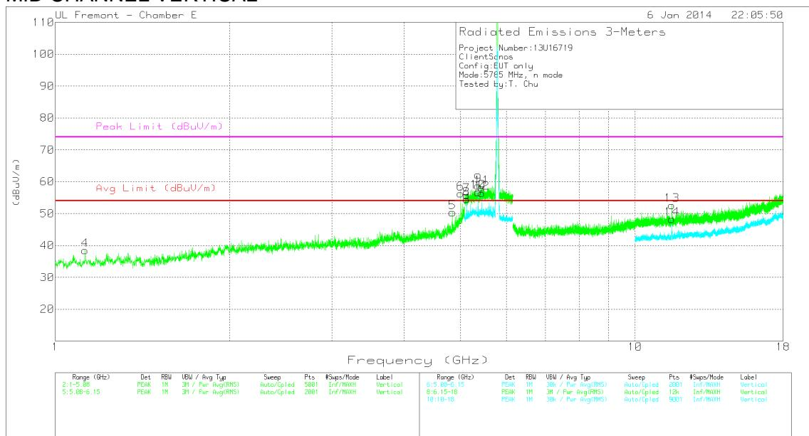
FCC Part15C All 5GHz UNII and DTS Spurious Emissions with Average Scan.TST 30915 4 Jan 2014
