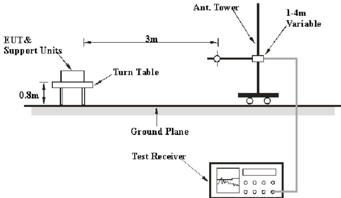
The radiated emission tests were performed in the open area 3-meter test site, using the setup accordance with the ANSI C63.4-2001. The specification used was the FCC 15.209 and 15.239 limits.
