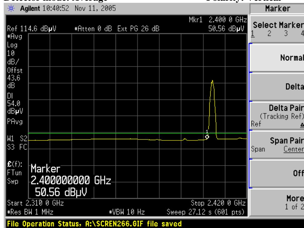
**Detector mode: Peak****Polarity: Horizontal**
