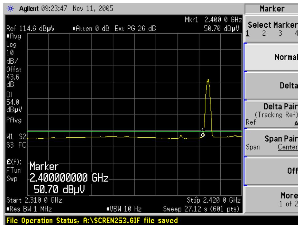
**Band Edges (CH High)****Detector mode: Peak****Polarity: Vertical**
