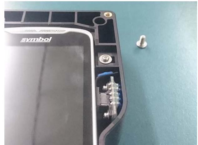
④ Place the cover and fix the screws (4 places) with the supplied screwdriver to complete mounting.
