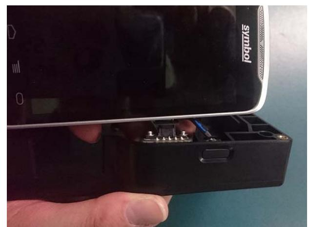
③ Please TC55 to be parallel with Outer case. In that state slowly push it into the Outer case with both hands. In addition, the USB cap of TC 55 will be put in the position of the picture on the right.
