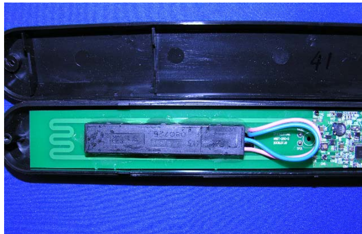
434MHz Antenna(PCB Loop Antenna) and 125kHz Antenna(Ferrite Bar Antenna) View
