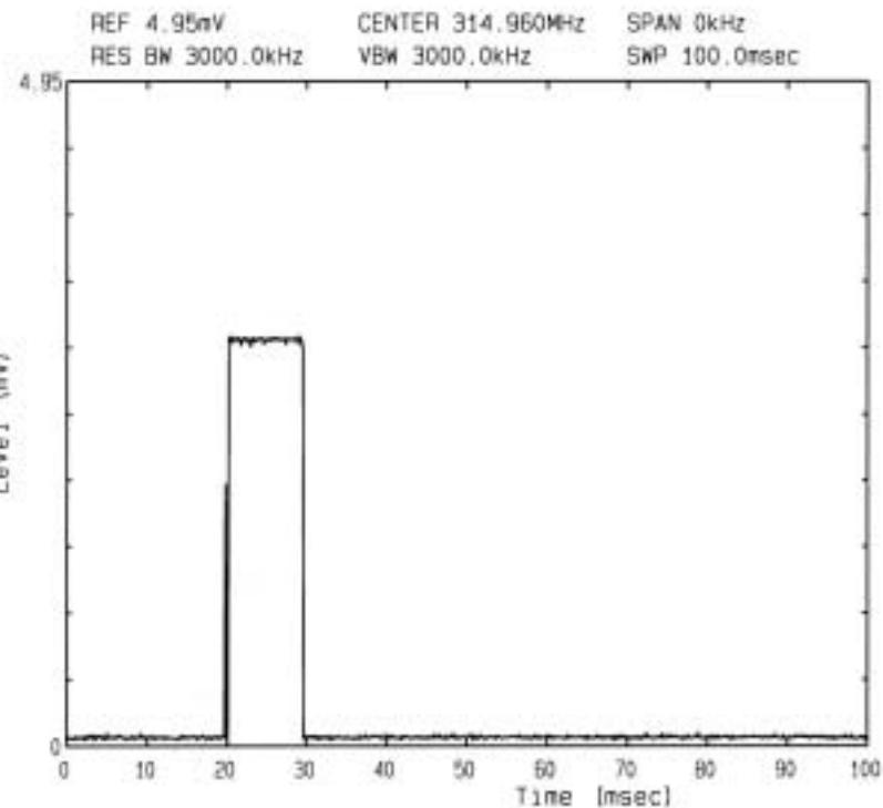
The above waveform indicates the case when field strength averaged over 100 milliseconds was maximum value.
