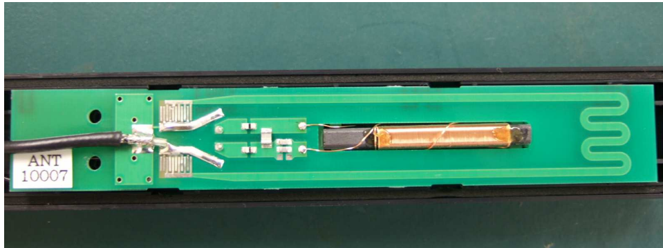
TOP View of ANTENNA PCB
