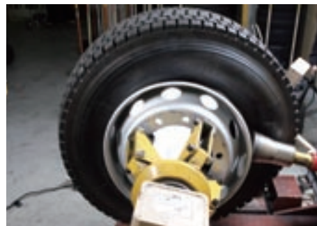
Remove the inner bead
