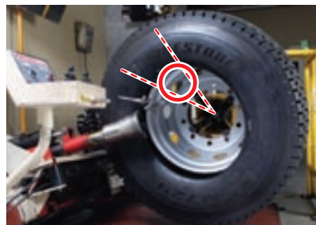
Valve is above the bead roller horizontal position (10 to 11 o'clock position)
