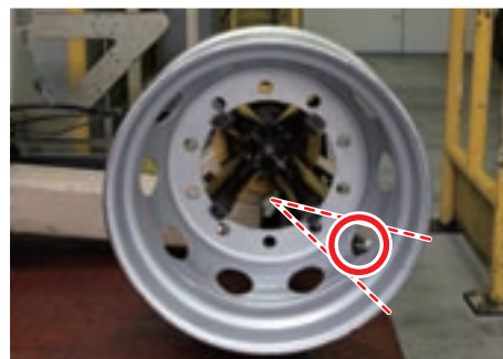
Valve is between 4 to 5 o'clock position.
