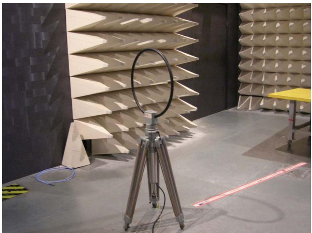
For radiated emissions 30MHz~1GHz
