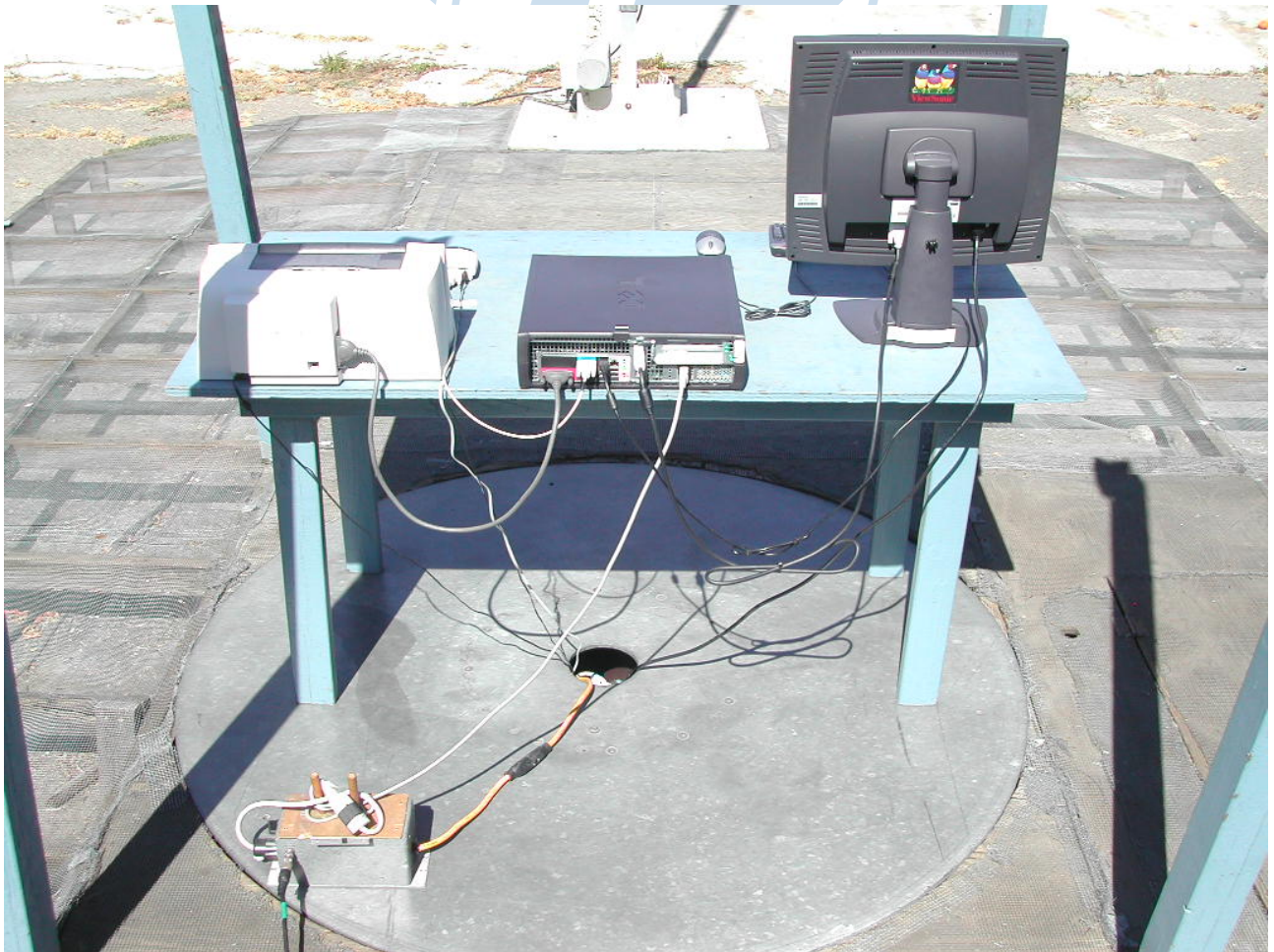
FIGURE 3: PLI Photograph Number 5397C2134SJR-01 illustrates the rear view of the host PC with all peripherals attached in Conducted EMI test configurations. The EUT is installed in the Personal Computer System.
