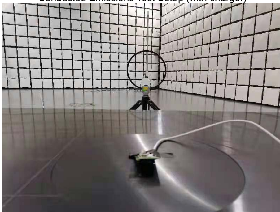
Conducted Emissions Test Setup (with charger)
