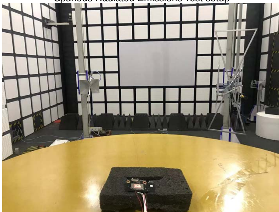
Spurious Radiated Emissions Test setup
