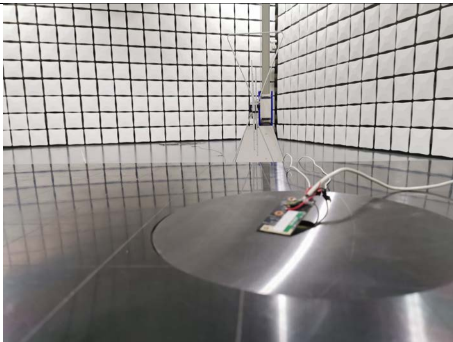
Spurious Radiated Emissions Test setup
