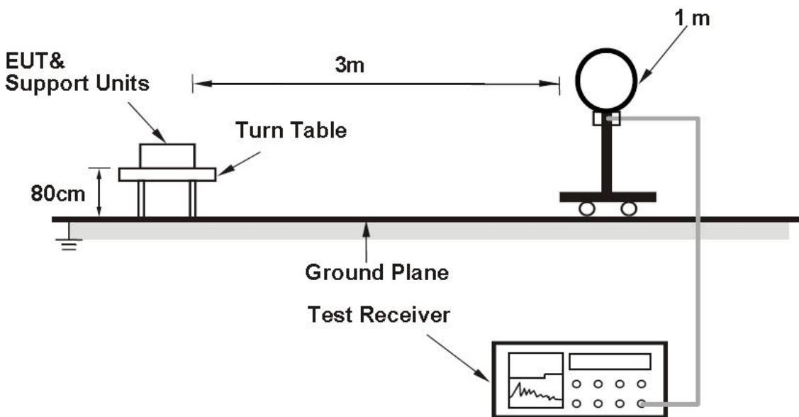
**For Radiated emission 30MHz to 1GHz**
