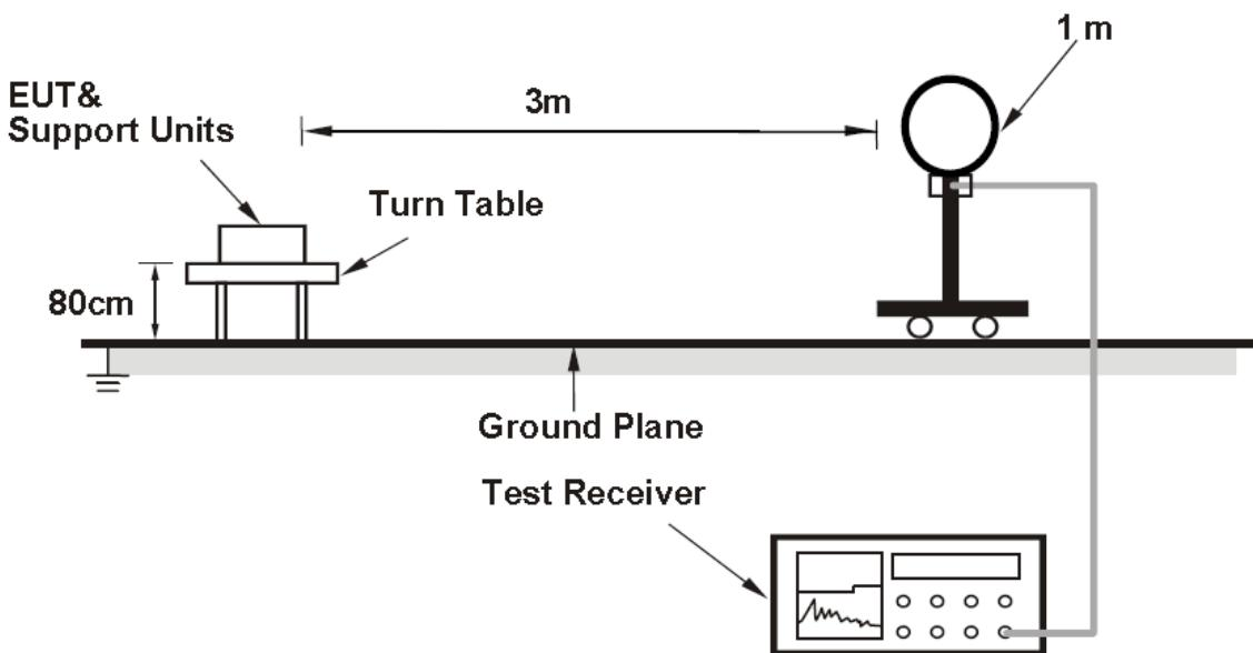
**For Radiated emission 30MHz to 1GHz**
