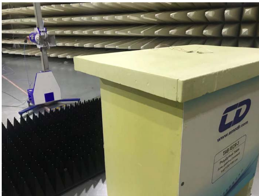
Spurious Radiated Emissions Test setup
