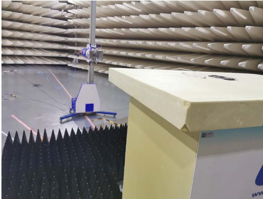
Spurious Radiated Emissions Test setup
