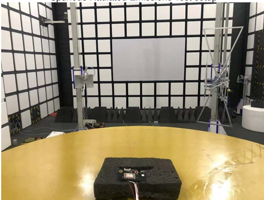
Spurious Radiated Emissions Test setup
