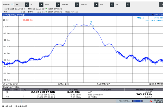
Figure 7.4-4: 6 dB bandwidth on low channel
