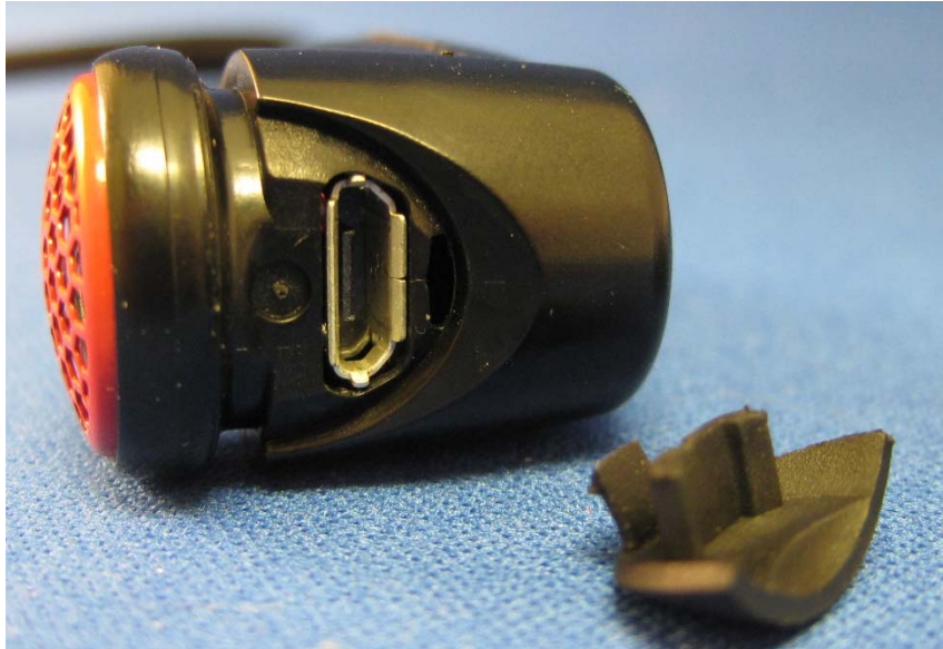
CLOSE-UP OF PORT USED FOR CHARGING
