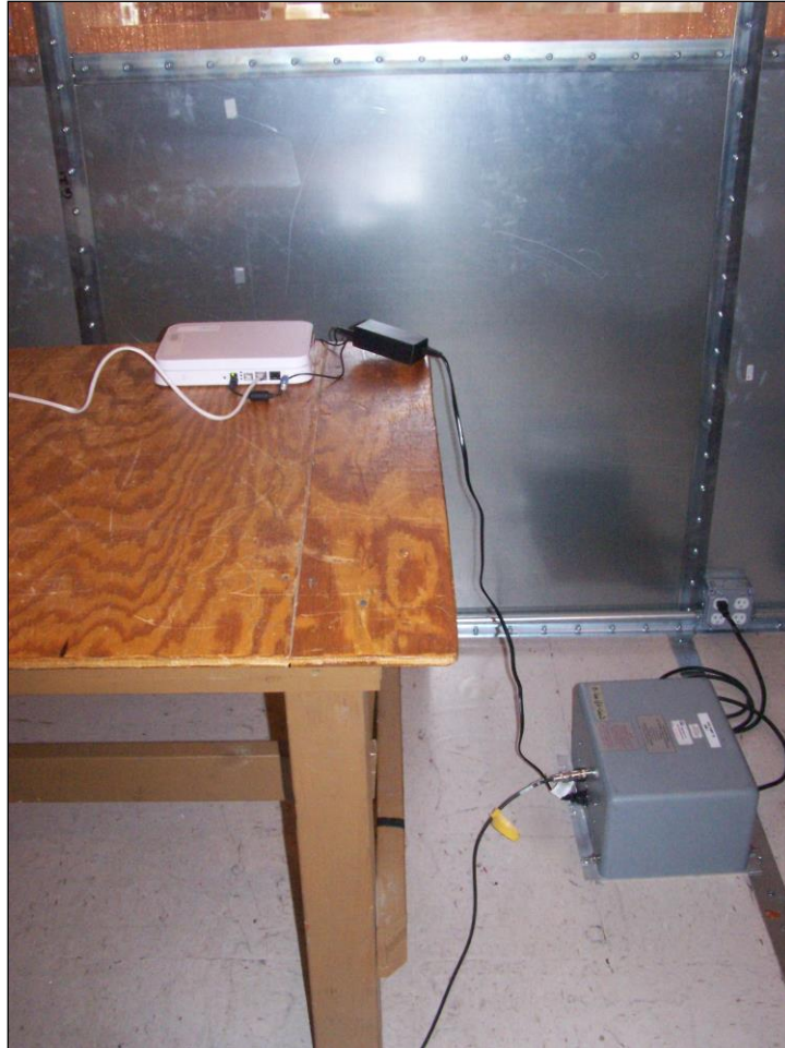
Photograph 3. Conducted Emissions, 15.207(a), Test Setup
