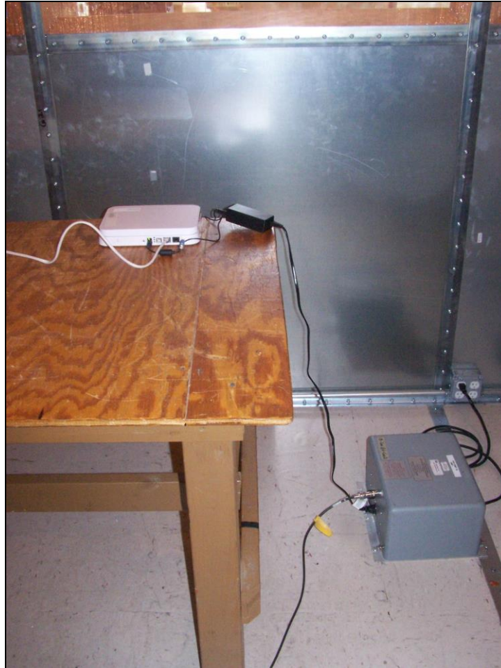
Photograph 2. Conducted Emissions, Test Setup
