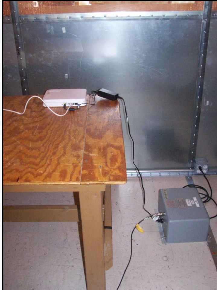
Photograph 4. Conducted Emissions, 15.207(a), Test Setup
