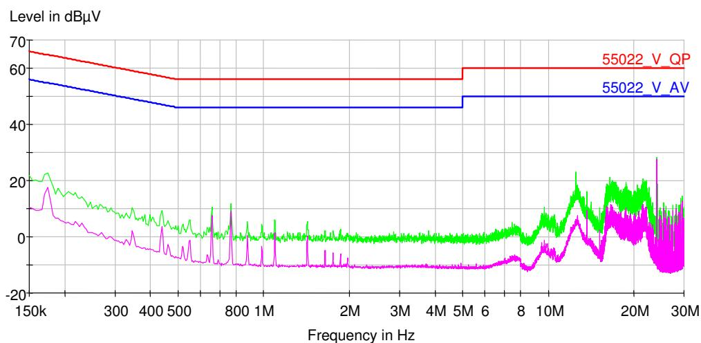
**150 kHz÷30 MHz – NEUTRAL LINE****Modulation: GFSK**
