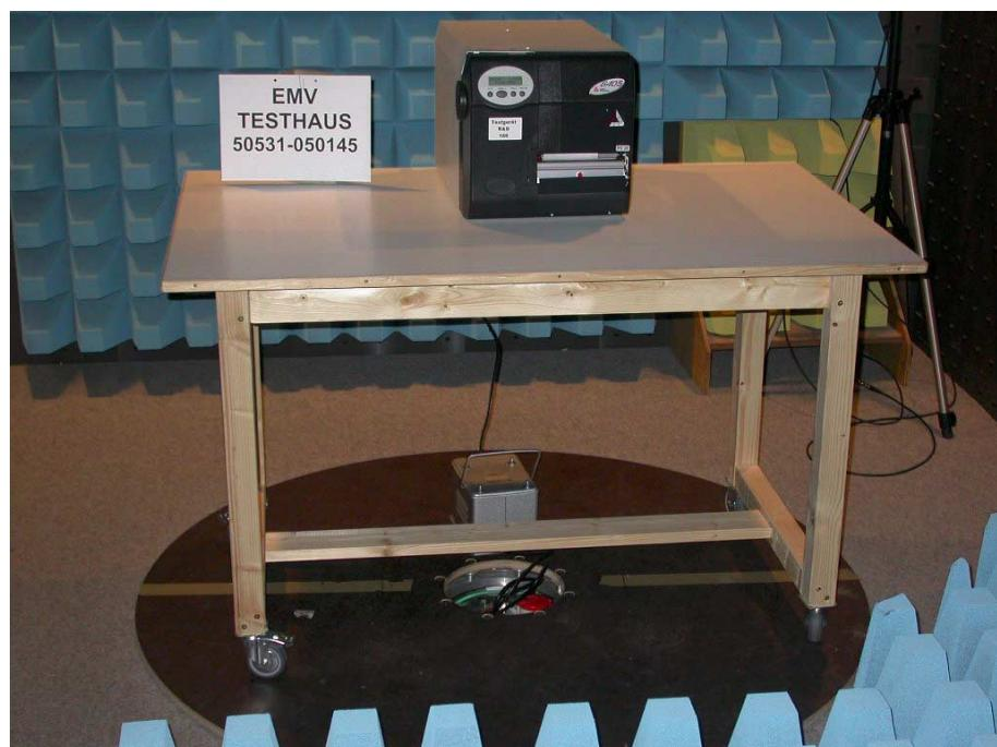
**Test setup for radiated emission measurement 30 MHz – 1 GHz
