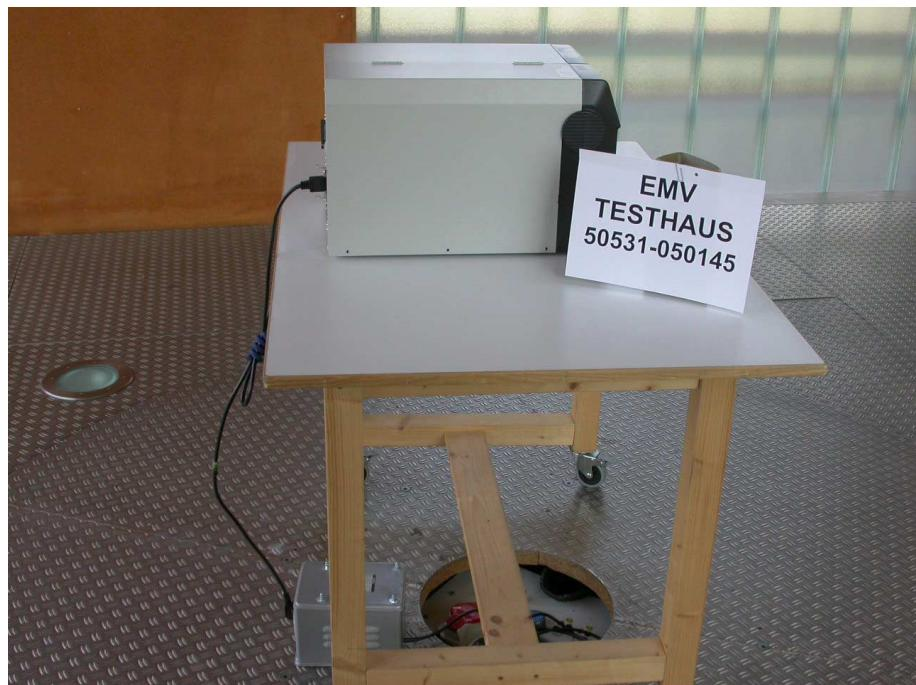
**Test setup for conducted AC Powerline Emission Mesurement**
