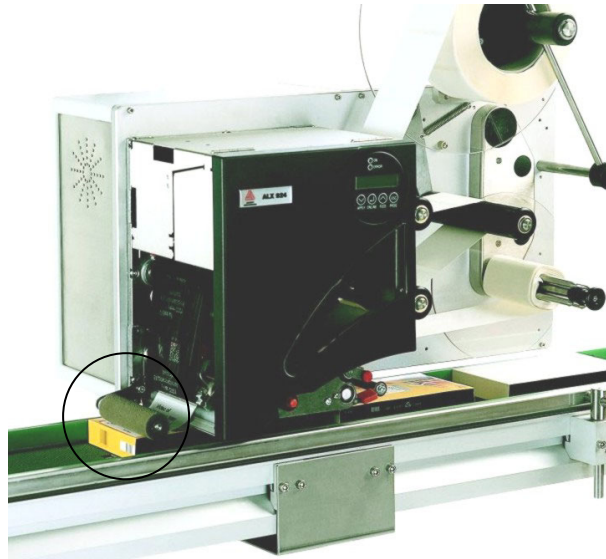
Fig. 9: The application roller presses the label onto the product directly after dispensing it.
