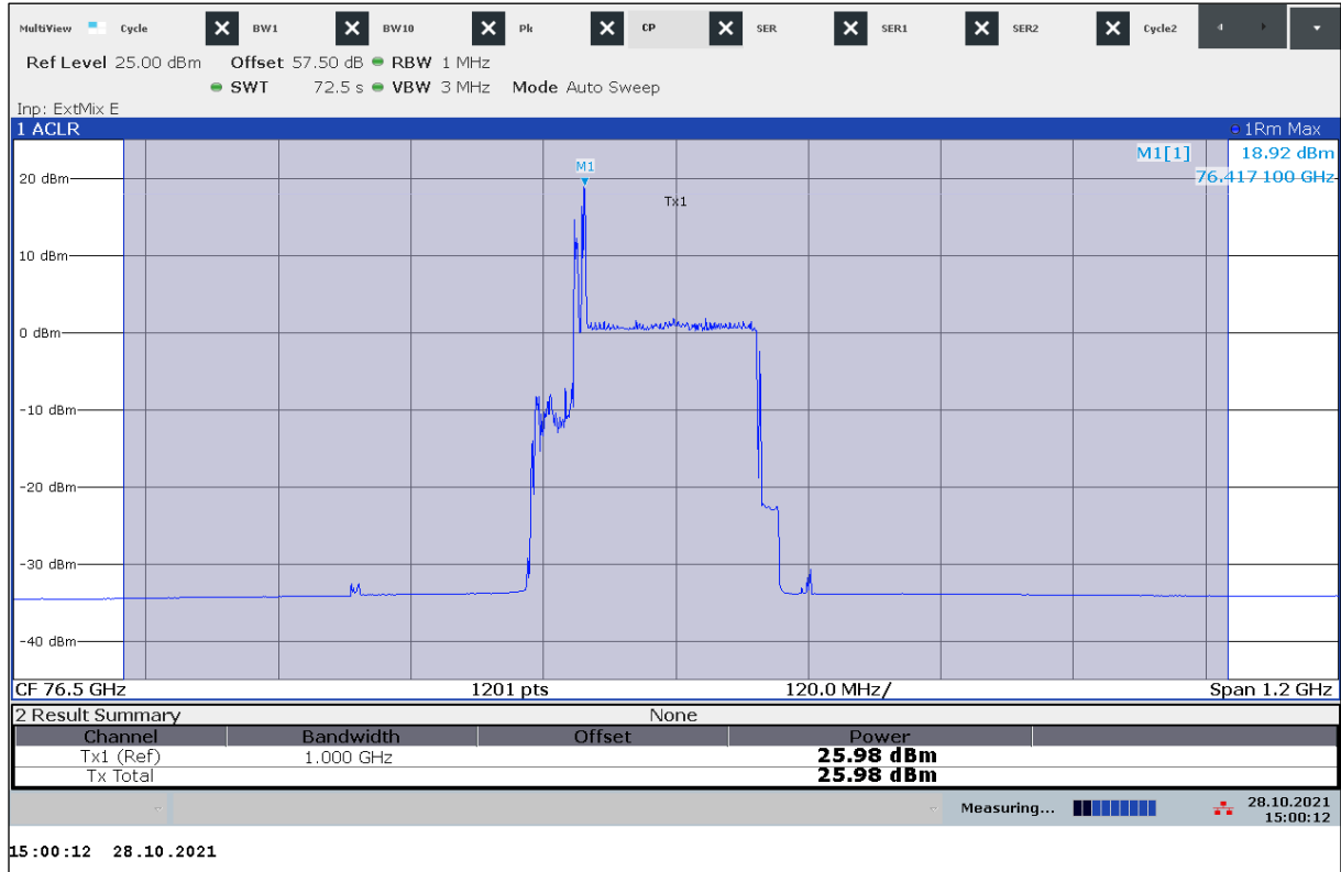
Plot 1: EIRP Mean Power (Channel Power), Long Range, T_{nom} / V_{nom}
