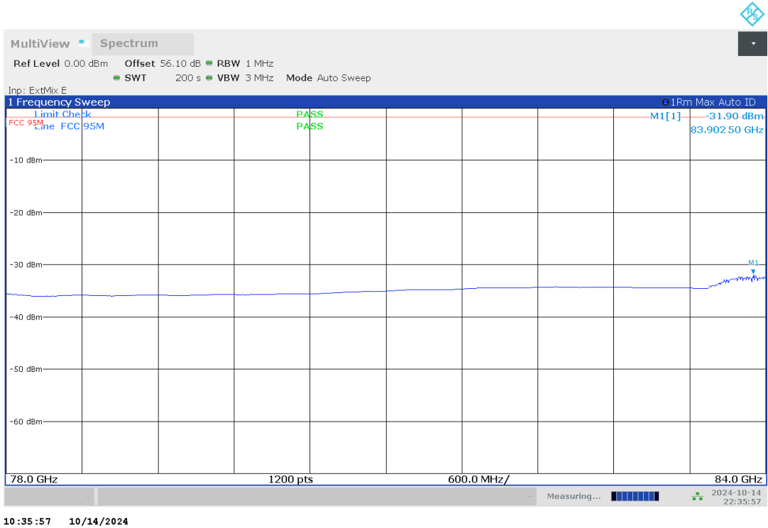
Plot no. 40: radiated emissions 78 GHz – 84 GHz, Mode 15, polarization vertical / horizontal
