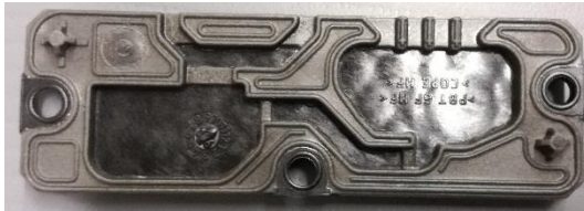
EMC shielding – internal view
