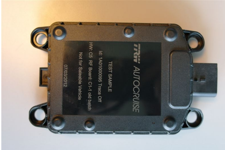
Figure 1: Rear view of the sensor, with the location for laser engrave information
