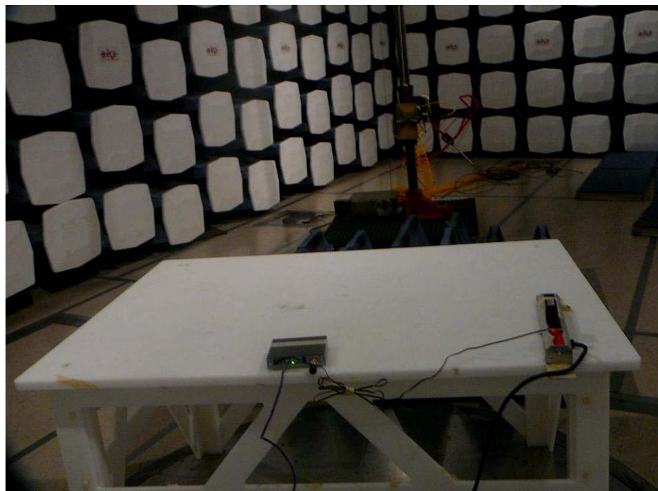
**15.11 RX Radiated Emission (POE Powered) Front View**
