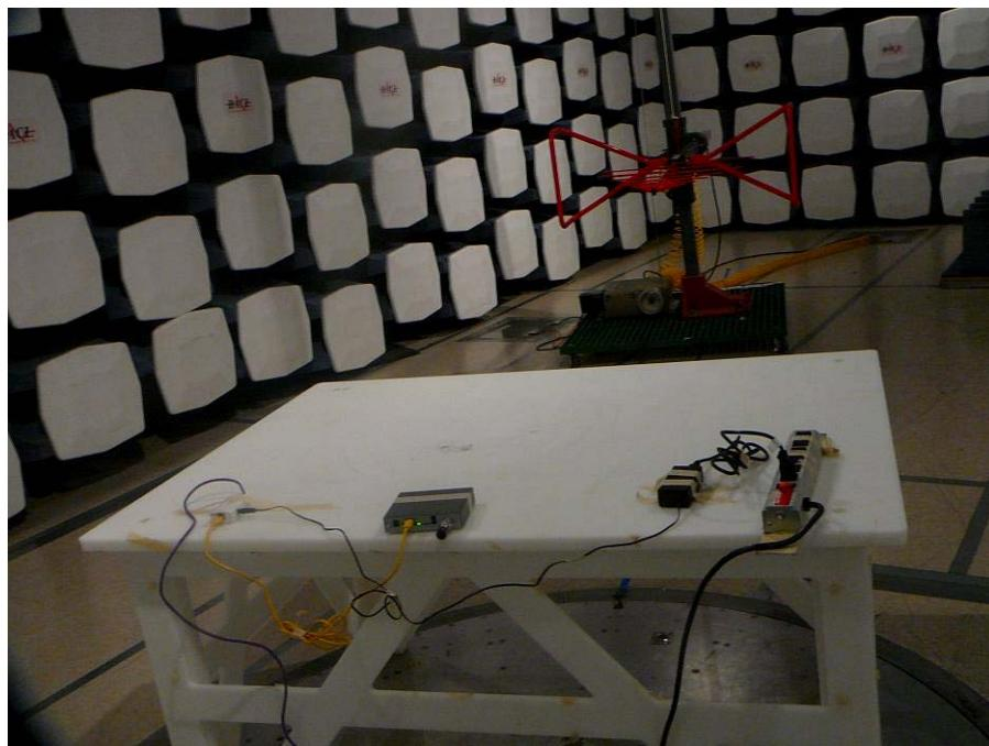
**15.13 RX Radiated Emission (POE Powered) above 1 GHz Rear View**
