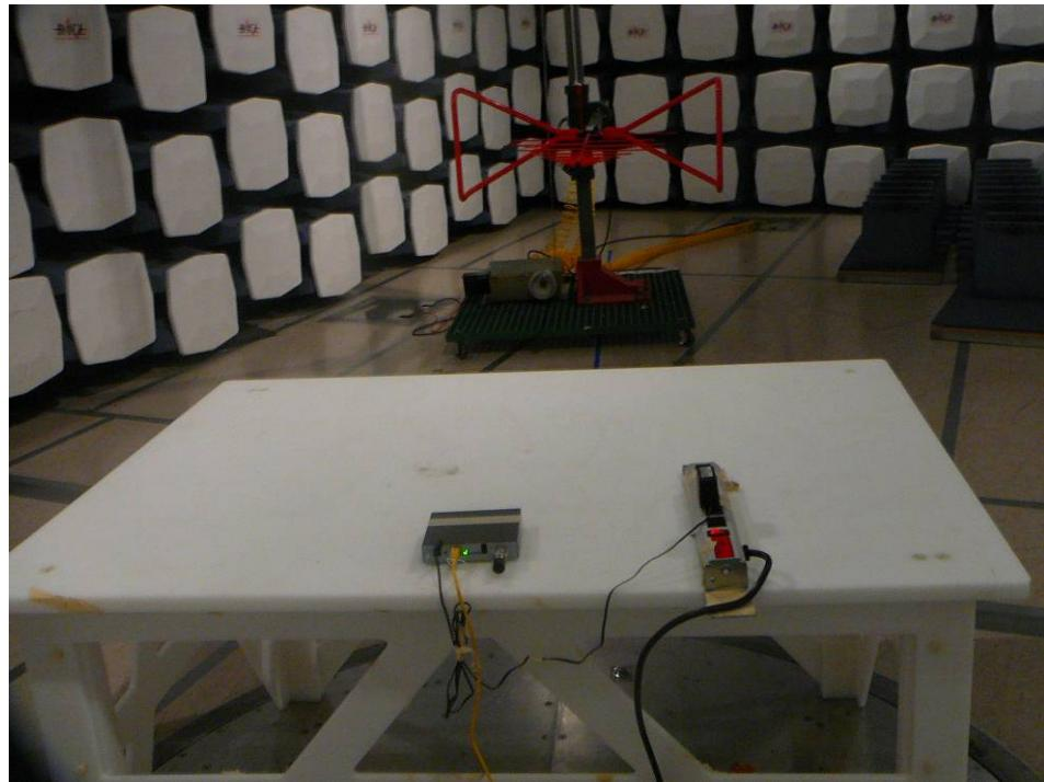
**15.10 RX Radiated Emission (AC/DC Adaptor Powered) above 1 GHz Rear View**
