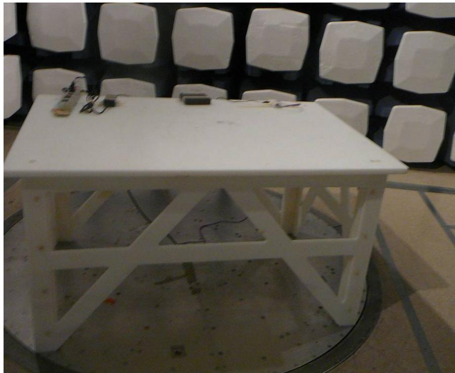
**15.12 RX Radiated Emission (POE Powered) below 1 GHz Rear View**
