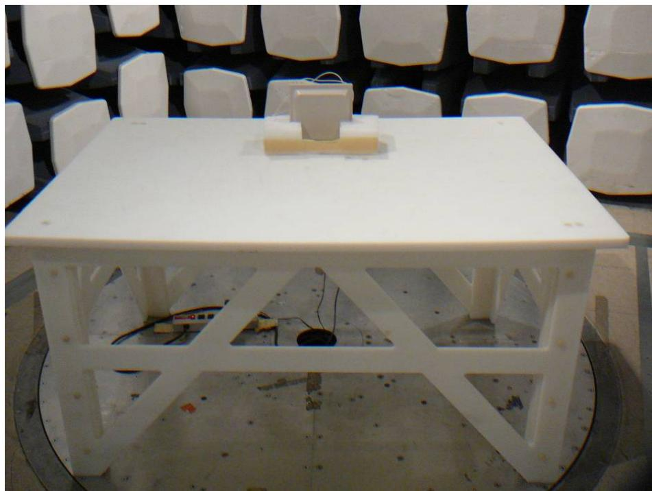
**16.12 Radiated Emission below 1 GHz Rear View (7.5 dBi Patch Antenna)**
