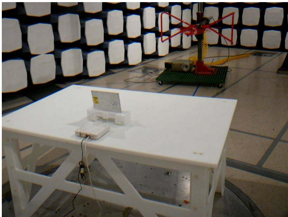
**16.10 Radiated Emission above 1 GHz Rear View (5 dBi Patch Antenna)**
