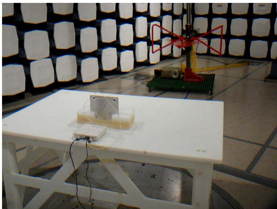
**16.13 Radiated Emission above 1 GHz Rear View (7.5 dBi Patch Antenna)**
