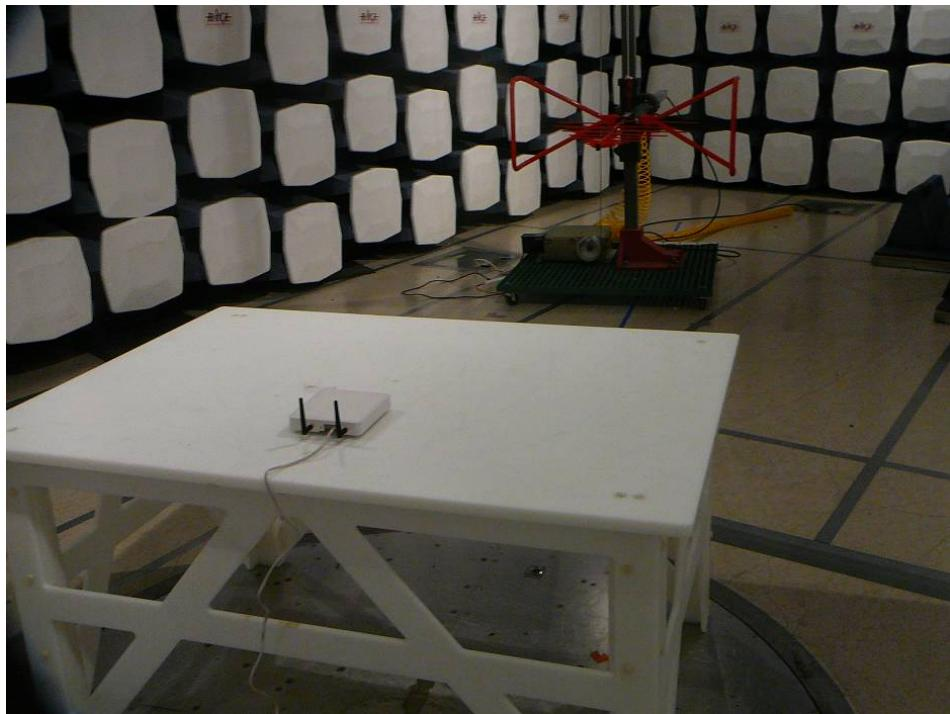
**16.7 Radiated Emission above 1 GHz Rear View (Dipole Antennas)**
