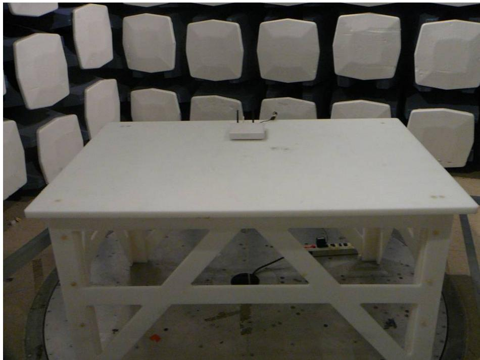
**16.6 Radiated Emission below 1 GHz Rear View (Dipole Antennas)**
