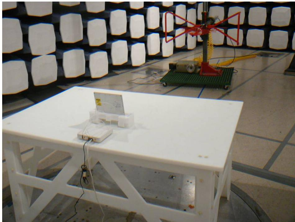
**16.10 Radiated Emission above 1 GHz Rear View (Patch Antenna)**
