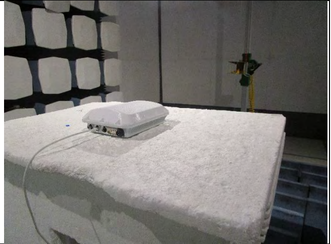
Radiated Emissions (>1GHz) – Rear View
