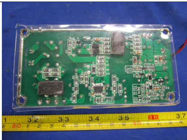
EUT Internal Power Distributor – Solder View
