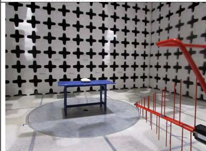
Radiated Emissions (<1GHz) – Front View
