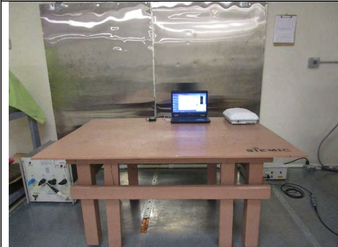
AC Line Conducted Emissions – PoE – Front View
