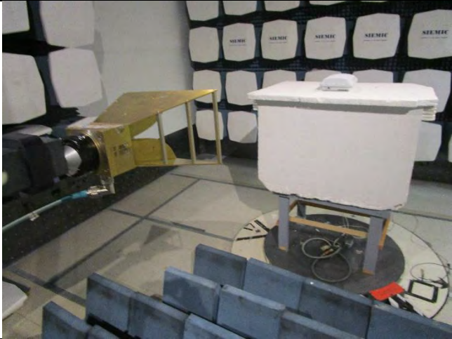
Radiated Emissions (>1GHz) – Front View
