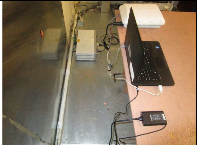
AC Line Conducted Emissions – PoE – Rear View
