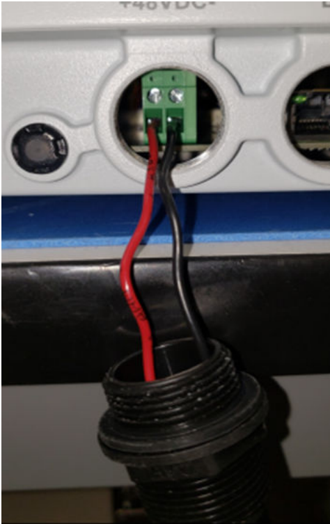
FIGURE 7 Connecting DC Wires To Terminal Block
