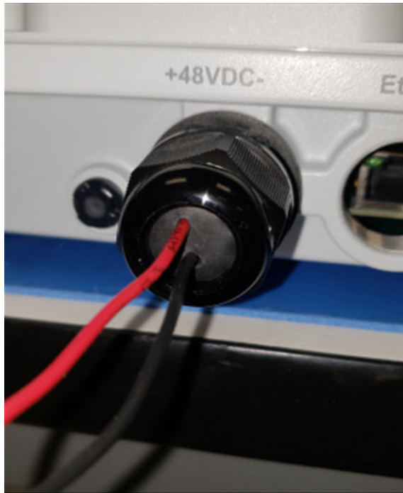
FIGURE 10 Tightening the Cable Gland Dome
