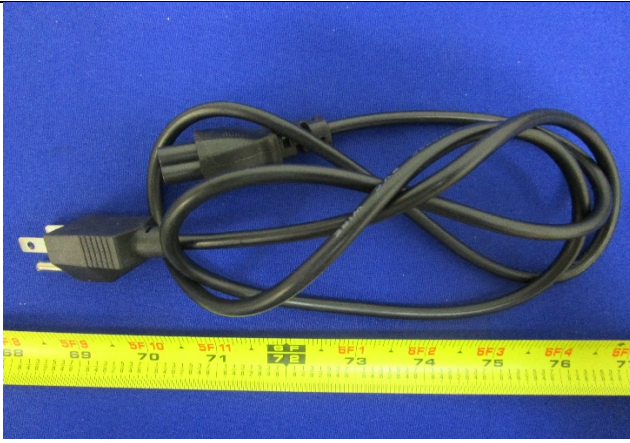
EUT AC Line Power Cord
