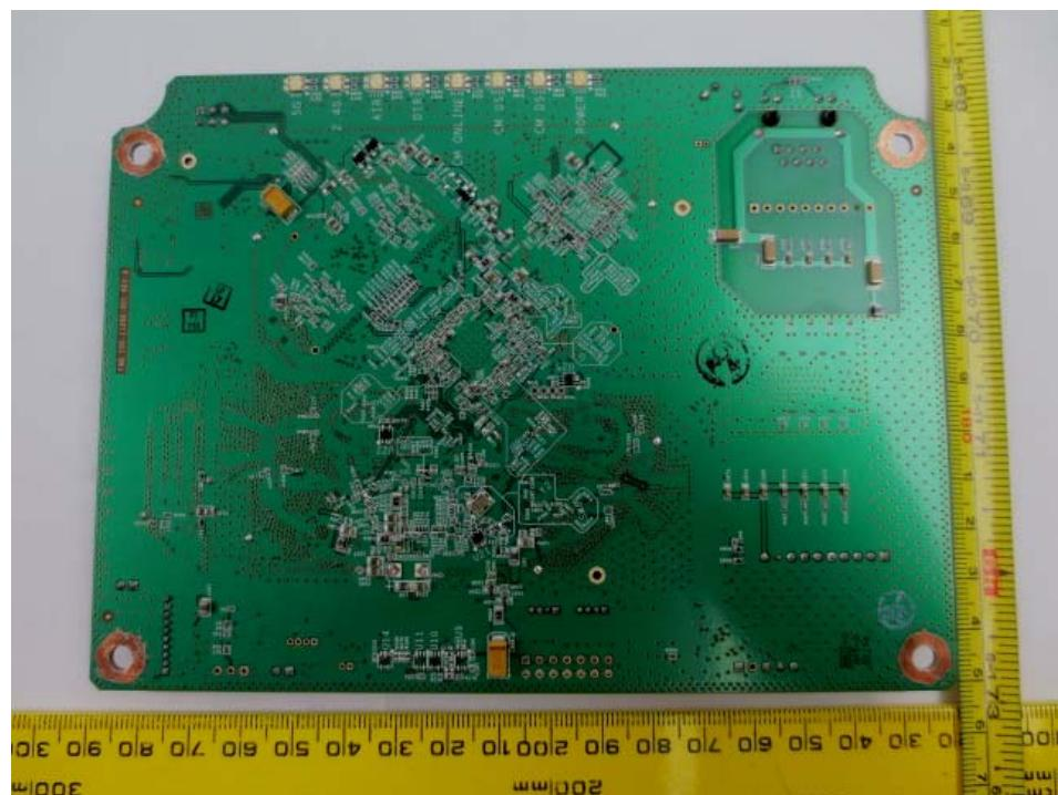
**14.13 Main Board Shielding off View**
