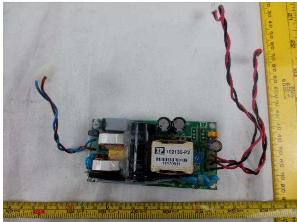
**14.17 Power Supply Board Rear View**
