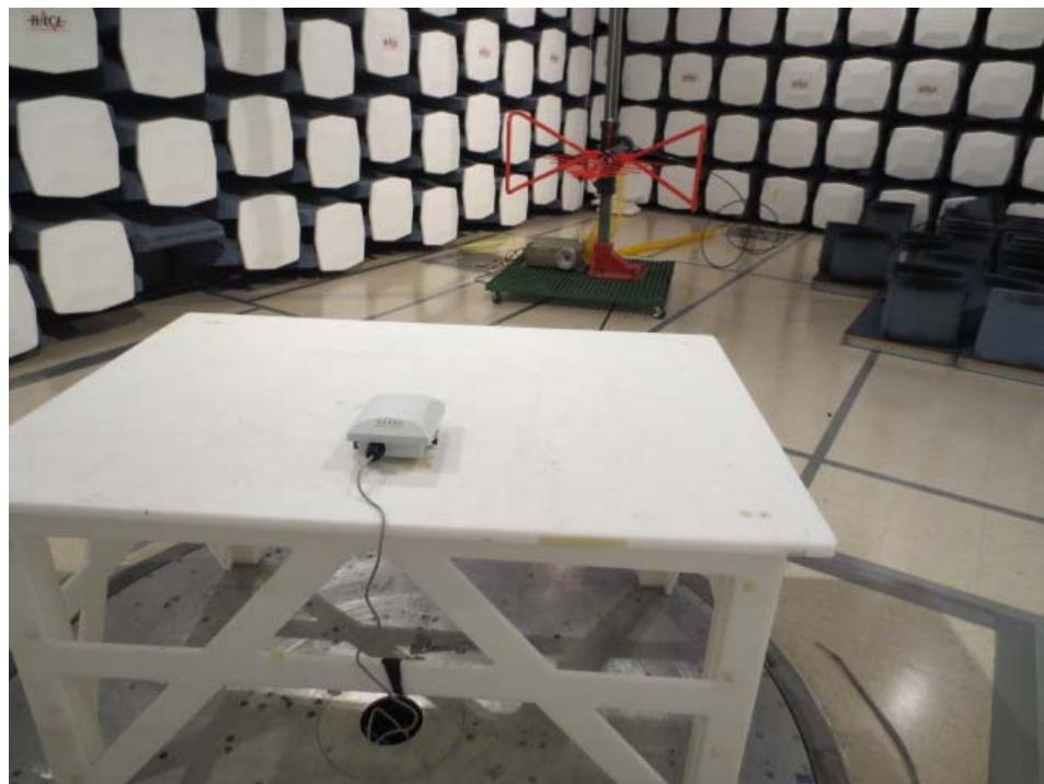
**13.5 Radiated Emission above 1 GHz Front View**
