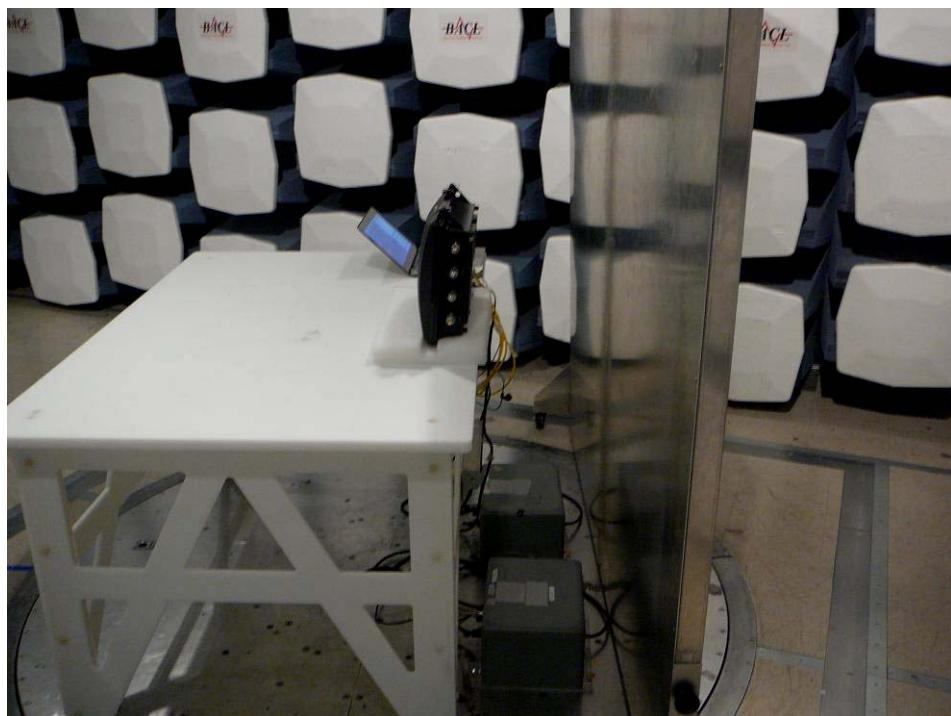
**16.3 Conducted Emissions POE Powered Front View**
