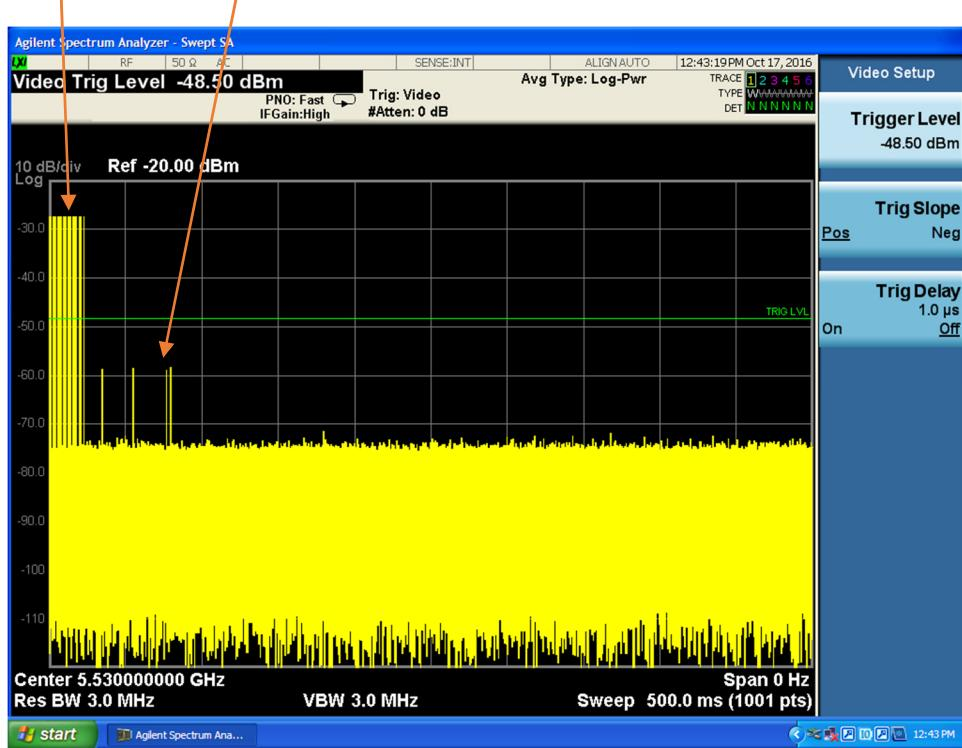
EUT have stream before radar signal detect.
