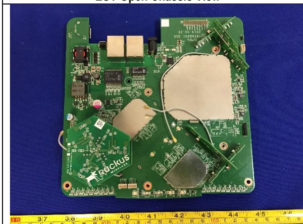
EUT Main Board - Top View with shielding
