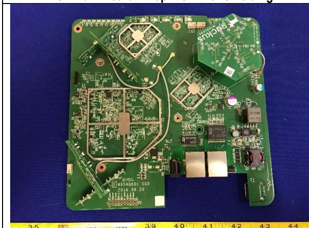
EUT Main Board - Top View without shielding
