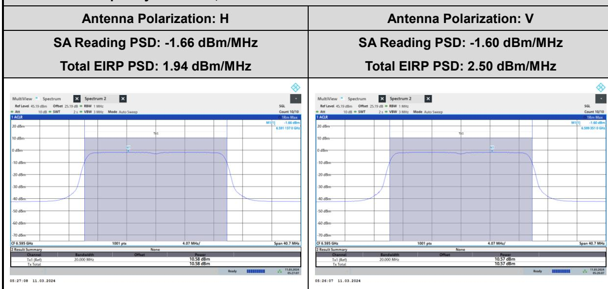
**LPI Mode FCC EIRP PSD Limit 5 dBm/MHz**
