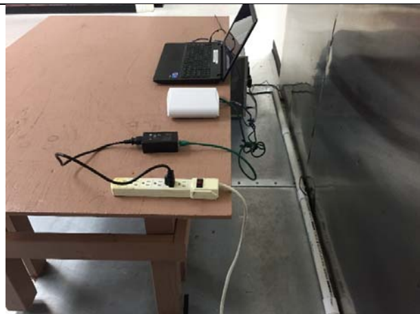
AC Line Conducted Emissions – Rear View
