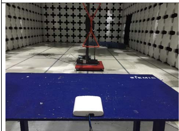
Radiated Emissions (<1GHz) – Front View
