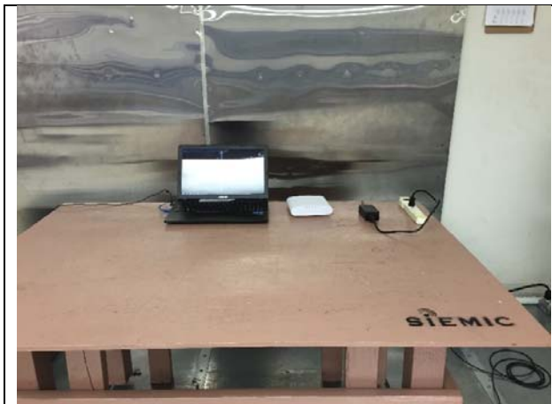
AC Line Conducted Emissions – Front View
