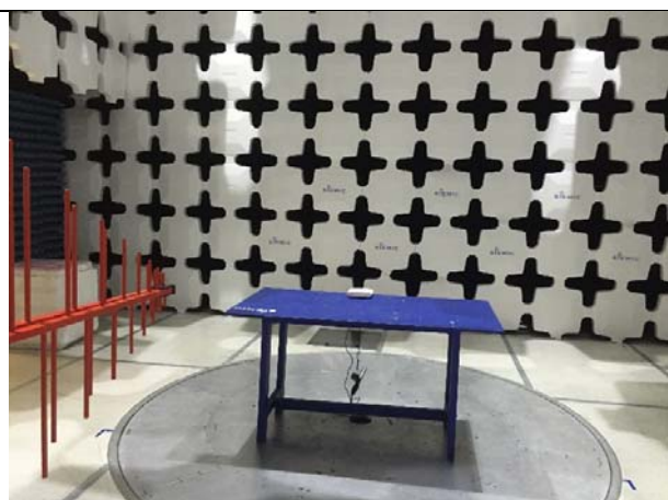
Radiated Emissions (<1GHz) – Rear View
