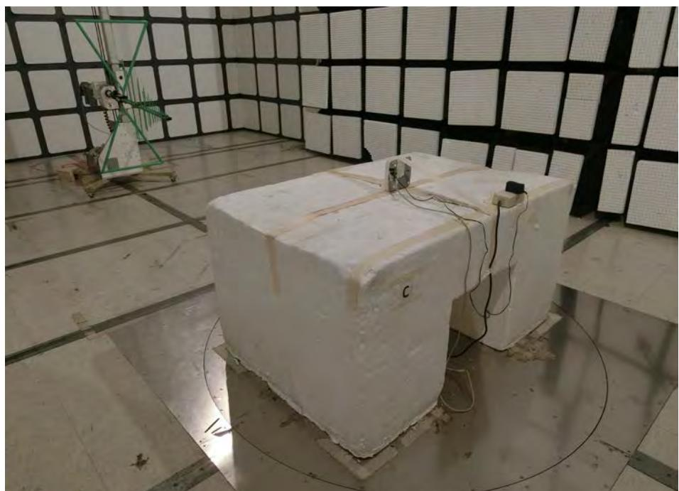
**Test Configuration: Above 1GHz****For Harmonic:****FRONT VIEW**
