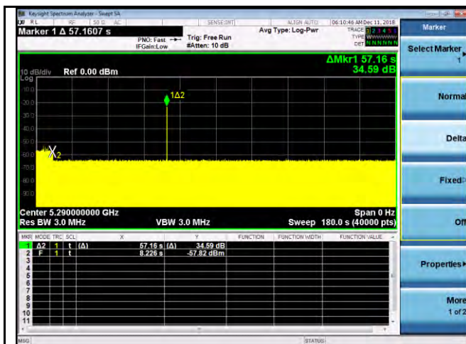
Radar at beginning of CAC – VHT80 – 5290MHz
