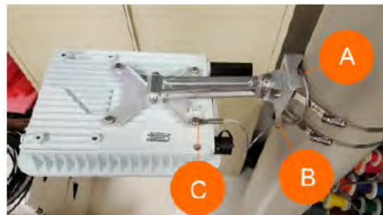
FIGURE 13 Attaching the Security Cable
